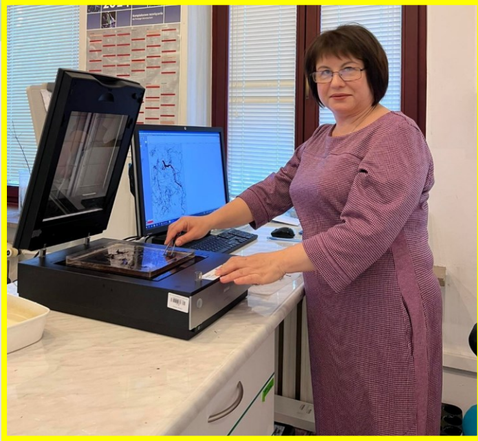
(Left) Dr Valentyna Dyshko scanning the roots of 2-year-old beech seedlings to assess possible damage to the fine roots. The plants were exposed to water stress and some of them received foliar treatment with the silicon preparation OPTYSIL MICRO in different doses. The water scanner and the WinRhizo software help to understand the protective role of silicon (Si).
