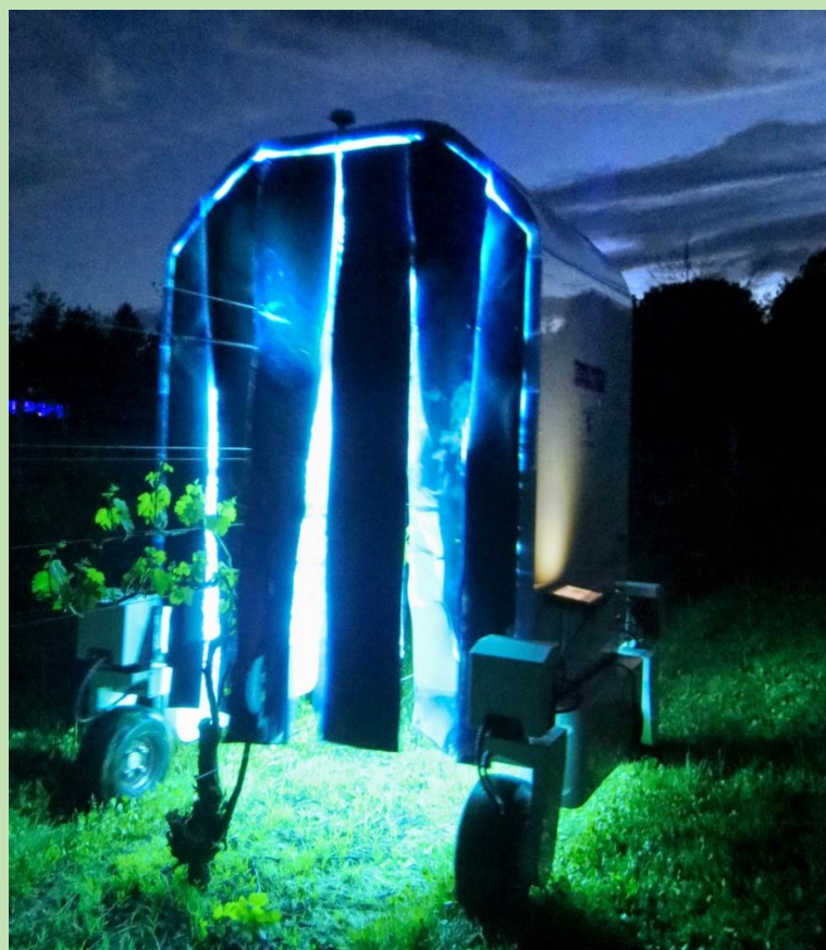
The UV light robot named Thorvald, applies treatment on grape vines in a Cornell AgriTech research field at night (Photo credit: David Gadoury, Cornell Agritech).
